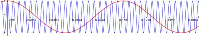
This time, we don't simply multiply the baseband signal to the carrier (as in AM). Instead, we "compress" and "stretch" the carrier (ie, modulate its frequency) based on the baseband signal.
