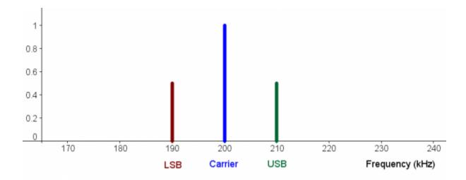
All this is saying is that the radio signal is composed of three pieces: a signal at 190 kHz with an amplitude of 0.5, a signal at 200 kHz with an amplitude of 1, and another at 210 kHz with an amplitude of 0.5.
