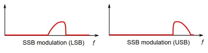
The two main advantages of using SSB (LSB or USB) are that:
