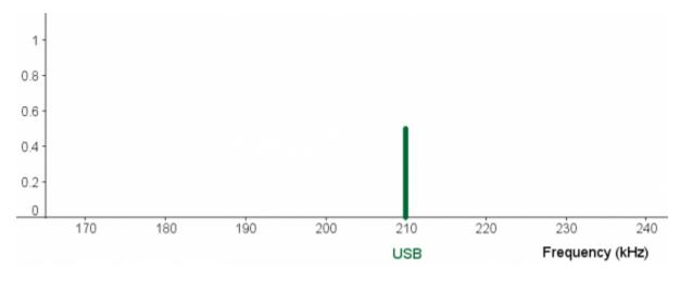
By itself, neither of these transmissions would carry the information we need (that the baseband signal was a 10 kHz note) since it's the difference between the sideband and the carrier that gives us that information. But if the receiver knows that this signal was generated by a transmitter at a frequency of 200 kHz, then the receiver can reinject the missing carrier on its side.
