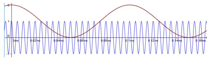
Finally, we **multiply** the envelope and the carrier, which gives us a wave that has the same frequency as the carrier, but an amplitude that varies like the voice signal:
