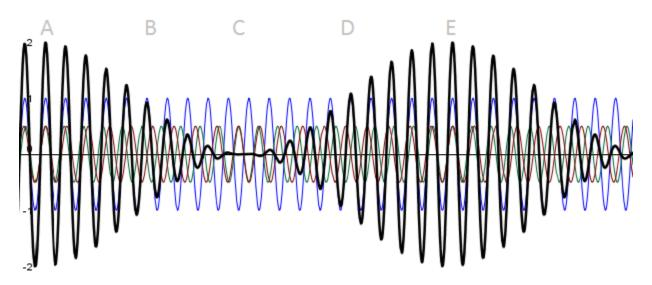
Note that the carrier as a frequency of 200 kHz just like the original carrier, but the two side bands are 10 kHz lower and higher with half of the amplitude. Notice also how the LSB Wave oscillates slower than the Carrier Wave, while the USB Wave oscillates faster.
