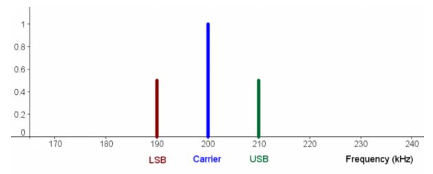
All this is saying is that the radio signal is composed of three pieces: a signal at 190 kHz with an amplitude of 0.5, a signal at 200 kHz with an amplitude of 1, and another at 210 kHz with an amplitude of 0.5.
