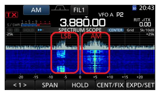
The radio is tuned to 3.880 MHz (where no one is transmitting), but there are two different conversations going on: one at 3.875 MHz using LSB, and another at 3.885 MHz using AM. The scope shows the recent history of the radio signal (called *waterfall*) where the present is at the top and the past at the bottom. Blue represent a weak signal strength and yellow or red represent a strong signal strength. Here are some things to notice:
