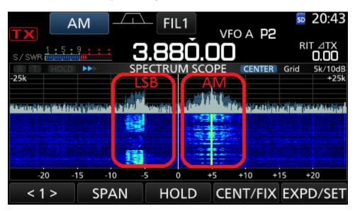
The radio is tuned to 3.880 MHz (where no one is transmitting), but there are two neighbouring conversations going on: one at 3.875 MHz using LSB, and another at 3.885 MHz using AM. The scope shows the recent history of the radio signal (called *waterfall*) where the present is at the top and the past at the bottom. Blue represent a weak signal strength and yellow or red represent a strong signal strength. Here are some things to notice:
