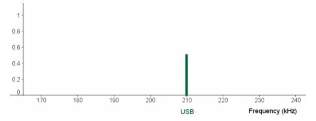
By itself, neither of these transmissions would carry the information we need (that the baseband signal was a 10 kHz note) since it's the difference between the sideband and the carrier that gives us that information. But if the receiver knows that this signal was generated by a transmitter at a frequency of 200 kHz, then the receiver can reinject the missing carrier on its side.
