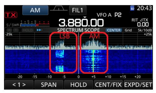
The radio is tuned to 3.880 MHz (where no one is transmitting), but there are two neighbouring conversations going on:
