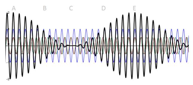
Note that the carrier as a frequency of 200 kHz just like the original carrier, but the two side bands are 10 kHz lower and higher with half of the amplitude. Notice also how the LSB Wave oscillates slower than the Carrier Wave, while the USB Wave oscillates faster.
