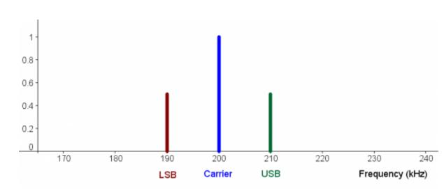
For example, the spectrum of our 10 kHz note transmitted over a 200 kHz carrier would look like this:
