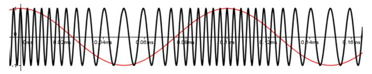
Here, the math is a bit more involved and requires at least  $1^{st}$  year calculus to understand but in a nutshell, if the carrier is  $\s c(t) = \cos(2 pi f_c t)$  and the baseband signal is  $\s t(t)$ , then the FM signal will be:
