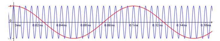
With the radio carrier frequency several times greater than the baseband audio signal.
