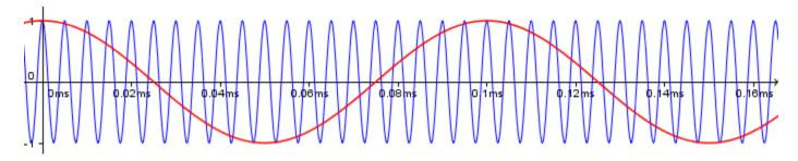
With the radio carrier frequency several times greater than the baseband audio signal.
