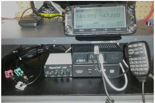
I use a short audio cable extension so that I don't have to reach behind the radio to connect and disconnect the speaker or SignaLink cable, and I ziptied the SignaLink patch cord (white) to the mic cord (black) so that they're easy to swap. Next, I'd like to get some sort of an A/B switch to easily select the Signalink or the external speaker.
