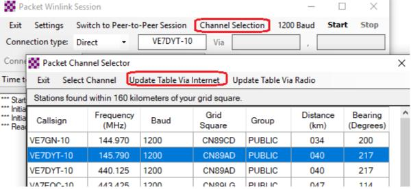
Once the table is updated, select an RMS near you, and ensure that the frequency of your radio matches that of the RMS listed in the table and press **Start**. At this point, two things will happen:
