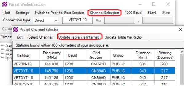
Once the table is updated, select an RMS near you, and ensure that the frequency of your radio matches that of the RMS listed in the table and press **Start**. At this point, two things will happen:
