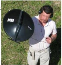
QRZNow published an article about the MFJ-5008, an ultrasonic receiver with parabolic dish that's "tuned to the ultrasonic range of 40 KHz allowing you to hear the ultrasonic noise generated by the corona discharge and arcing connections that generate the power line static on your radio." If anyone gets one, please report back on its efficacy.
