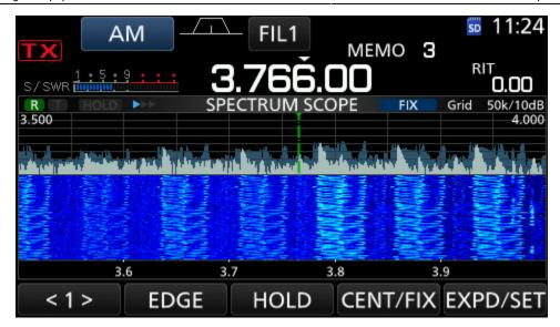
I offered to do a bit of research to see if the RFI could be filtered for their equipment. They told me they're using a Hilux Grow Light (AHS 1000) (a High Pressure Sodium Bulb) and a BCBallast (NL-HS1000/CGD2E) that I couldn't find any information about. Reading up a bit, it seems that it's the cheaper ballasts (not the bulbs) that are to blame for most of the RFI.
