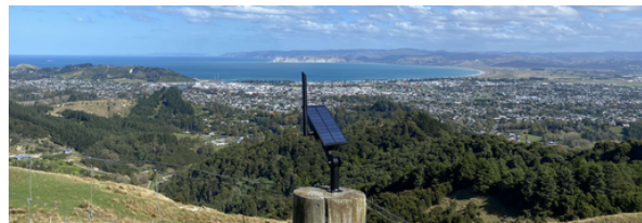
A MeshCore node setup as a repeater .
