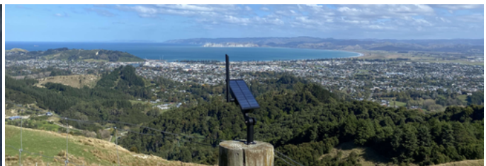
A MeshCore device setup as a repeater .
