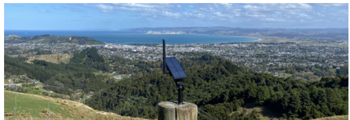
A MeshCore node setup as a repeater .
