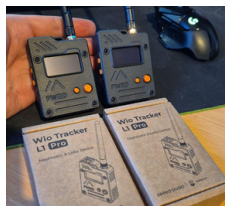
Two MeshCore nodes, often used as personal companion devices.
