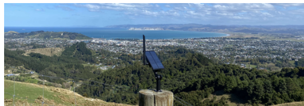
A MeshCore node setup as a repeater .
