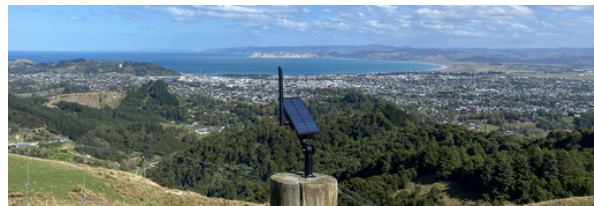
A MeshCore node setup as a repeater .
