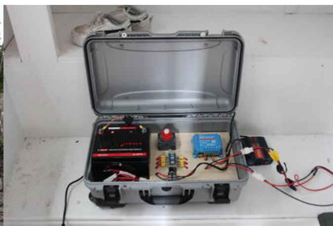
VE7LDB's solar battery box
