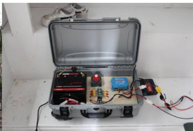
VE7LDB's solar battery box
